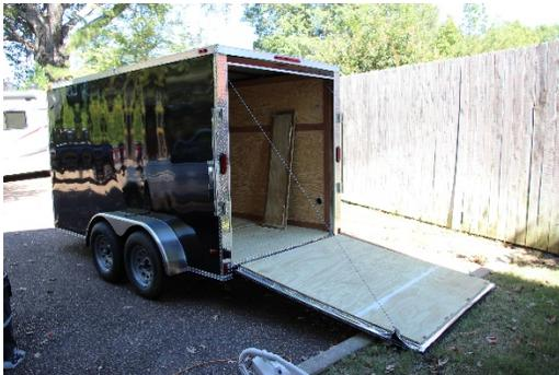
In the first step, a sealer – STAUF's VPU-155 S - was applied to all the plywood inside the trailer with a foam roller. This enables the second coat to stand up, and prevents penetration of the wood. This took 2 hours to properly dry before the next coat could be applied.
